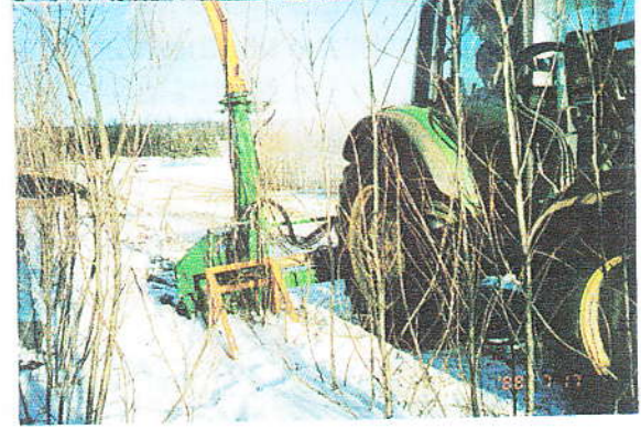
The JF-192 Harvester - Made in Brazil to harvest sugarcane, corn and some grasses for silage - Cost 35K - Mounts on a three point hitch.
