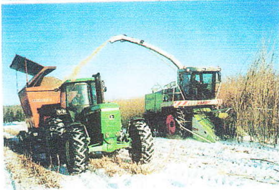
Claas Jaguar Silage harvester, with a modified cutting head for biomass production (willows) Made in Europe - Modified head alone costs 160K total cost unknown.
