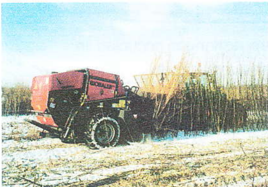
The Anderson Biobaler - Made in Quebec - for the purpose of harvesting all types of biomass Is used to remove growth in clearcuts, powerlines, pipelines etc -Cost 140K.
