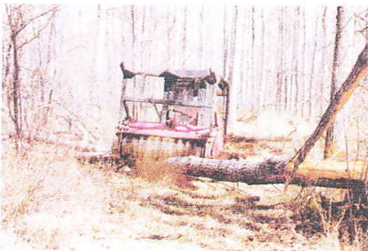
Figure 3 - Mulcher working its way through a large log
